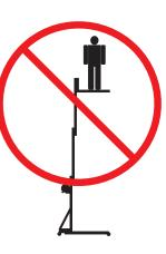
**NEVER** operate the material lift unless the legs and stabilizers are fully lowered and locked and all casters are in contact with the ground.
