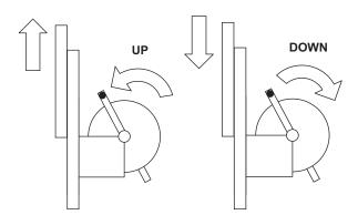
After lowering the load to the desired position, rotate the winch handles one quarter-turn toward the mast - as if raising the carriage - to set the brake
