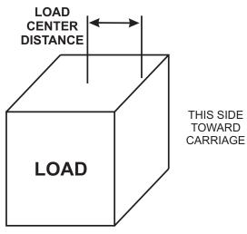
**NOTE:** Load center refers to the center of gravity of the load and may not be its physical center. The heaviest side of an uneven load should always be positioned closest to the carriage on the material lift.
