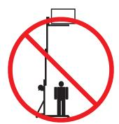
**NEVER** operate the material lift on a moving or mobile surface, such as a truck bed.
