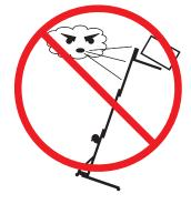
**NEVER** apply an additional side load or horizontal force to a material lift that is loaded or raised. **NEVER** place ladders or scaffold against the material lift.
