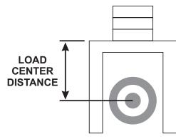
The load should be as close to the carriage as possible, and the load center should be centered between the forks
