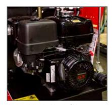
A powerful 13 hp Honda GX390 engine provides all the power and torque needed for any application.
